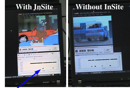
Fig. 12. Screenshot of a demonstration. Graphs showing stalls. Low point indicates a stall. Each dot indicates a 1 second stall. Client observes 3 stalls with InSite, and 6 stalls without InSite.
